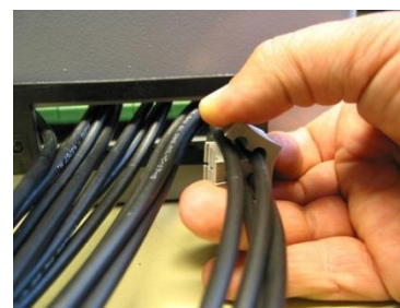
Figure 6-12 Clamp 4 cables into one insert
