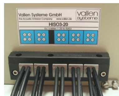
Figure 6-7 Front view on cable entry system (Ex i cables) and earth connection point
