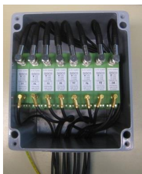
Figure 6-1 Top view into opened HISO3-08
