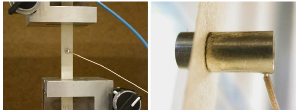
Fig. 2 Experimental setup and close up of the acoustic sensor
