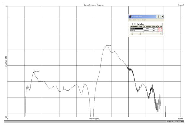
Source Crystal: Panametrics V101 / Source Voltage: Swept 60 - 750 kHz / Sweep Rep Rate = 14 mSec Input Signal VRMS = 0.141mV / Preamplifier: KRN BB-01 - 40dB
